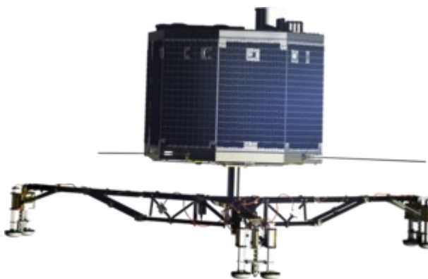
Figure 1: The Philae Lander consisting of a baseplate, an instrument platform, and a polygonal sandwich construction. The lander carries ten instruments, with a total mass of about 21 kilograms.
